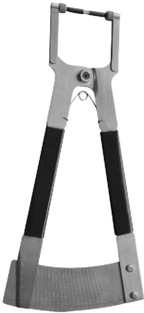
900-121 Wide Throat Lens Thickness Gauge Accommodates Lens Blanks Of Over 90mm Diameter & 22mm in Thickness. 47mm Throat Depth, 0.1mm Graduations. Overall Length 9-3/4"
