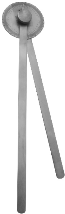
900-153 Protractor Goniometer Two Opposing 180 Degree Scales & One 360 Degree Scale, All Marked In 1 Degree Increments. Tension Between Arms Controlled By A Thumb Knob. 14" (35cm) Long
