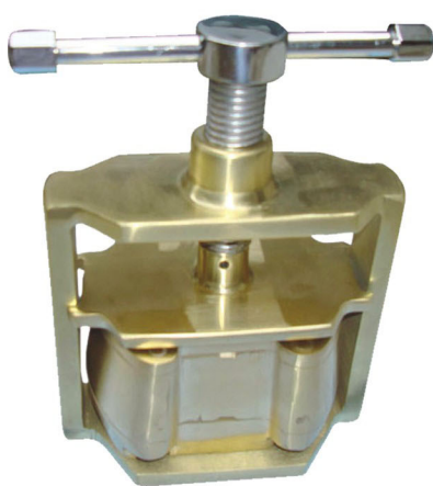
900-145-A Small Denture Flask & Bench Press Denture Flask Set Feature Forged Brass Alloy Construction. Fitted With Hardened Stainless Steel Alloy Rear Tapered Guide Pins. Flask Dimensions: 4" Long X 3 3/4" Wide X 2 1/4" High (10cm X 10cm X 6cm). Unit Weight: 2.425kg Including (flask & Bench Press)
